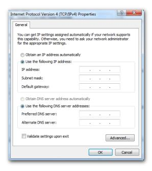
**Step 6 IP address, Subnet mask**: Set a static IP address, subnet mask for your computer, which is **192.168.0.10** and **255.255.255.0** in this example, and click **OK**.
