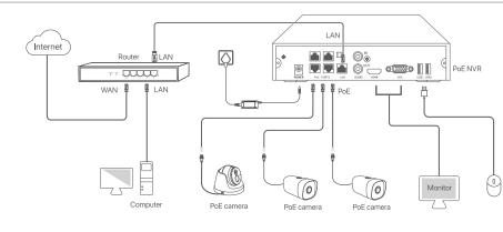
If the camera you want to add has been connected to the switch or router that is connected to the LAN port of the NVR, please ensure that the IP address of the camera and the NVR are in the same network segment.
